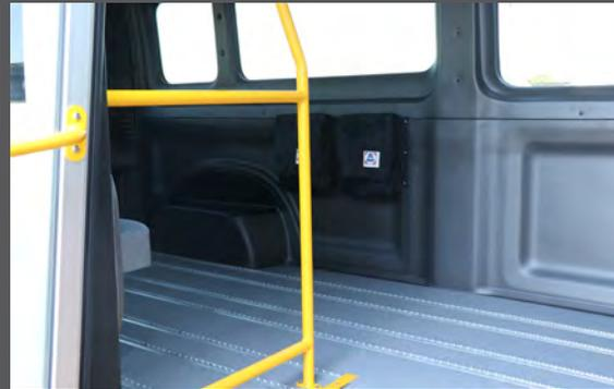
Extensive floor space for seating and securing wheelchairs and mobility devices.
